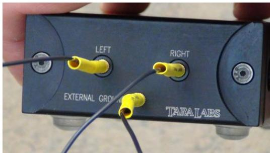
d) Once the #2 end of the mini Ground Lead is inserted into the component chassis, insert the #1 end of the mini Ground lead into the center input on the HFX station marked 'EXTERNAL GROUND.'
