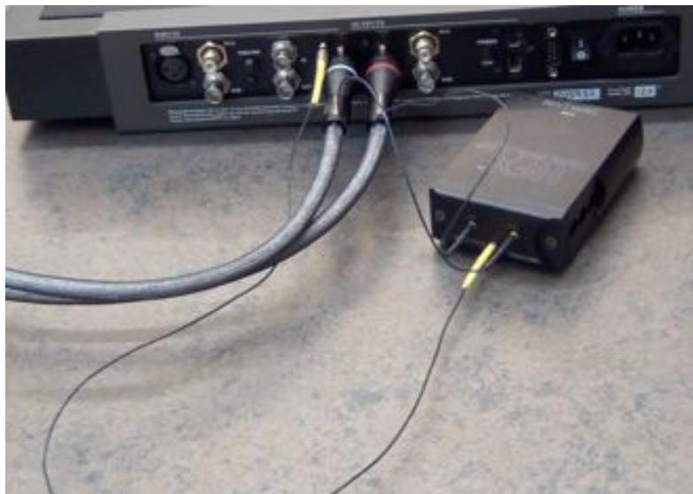
**TECHNOLOGY NOTE:** When combining the interconnects to the HFX Floating Ground Station, the Shield will be 'floated', not connected, to the circuit ground or (-) signal run of the cable. Instead, the HFX Floating Ground Station will provide an independent ground path and absorb RF/EMI energy in the shield, thereby lowering the noise floor for a much quieter cable as well as enhanced details.
