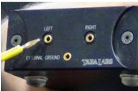
**Step 3:** Begin by inserting each Right & Left cable male mini-banana leads in to the HFX inputs marked 'RIGHT' and 'LEFT.'
