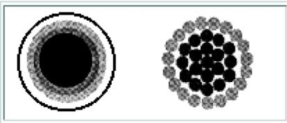
*Any compact or uniform shape increases the tendency of the whole conductor to have greater density in the coupling or linkage of electro-magnetic flux. In this diagram, a*
