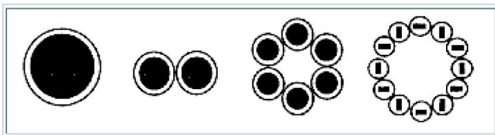
*All designs have the same conductive mass, but frequency linearity (i.e. a cleaner, clearer sound) will improve from left to right due to conductor size, shape & arrangement.*
